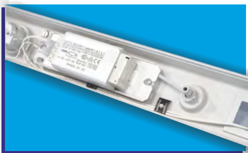
Low power factor (with magnetic ballast)
