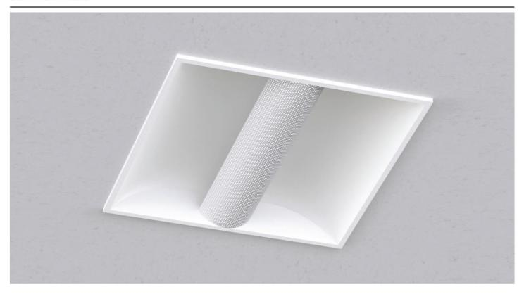
A recessed 600x600mm luminaire with special geometrical structure. The combination of the reflective recuperator and the micro-perforated lamp cover gives a direct-indirect light distribution, suitable for areas where soft, mostly indirect, illumination is required.
